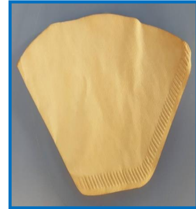
Bactericidal filter paper which can be used to remove bacteria in water
